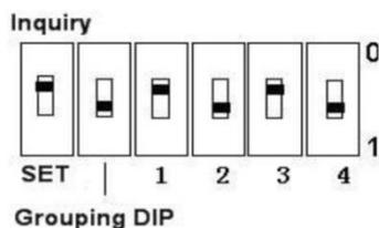
Settings can be configured by using the DIP Switches and the ▼,▲ buttons. To begin, the first DIP switch must be placed in position 1, and the required function entered on the remaining DIP switches. Press the 'V/A' button once and the display will flash. The value can now be adjusted using the ▼,▲ buttons. Press the V/A button once more to store the value.
