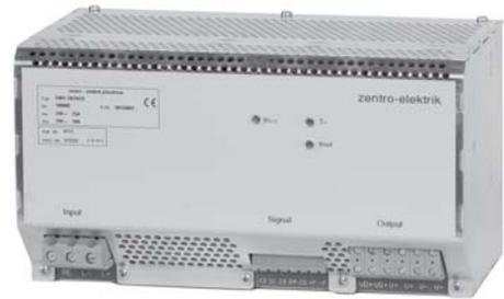
The GWH DC/DC - converter is designed for use in automation systems, power supply and power station engineering, traffic systems and mechanical and plant engineering. Cooling is provided by internal fans, all electrical connections are made using simple screw terminals, active current sharing takes place during parallel operation. As an option the product can be ruggedised to comply with EN50155 and 50121 for railway applications.
