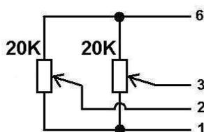
+5V output can be used to feed logic voltages for external circuits. Connection in an example works as a potentiometer controlled power supply. It is important to notice that +5V output is not allowed to load more then 20mA or proper operation is not guaranteed.
